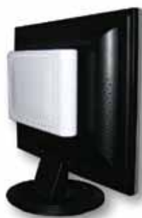
Figure 6: Thin client computer mounted on back of LCD monitor
